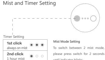
To switch between 2 mist mode, please press switch for 2 seconds until indicator blinks:
